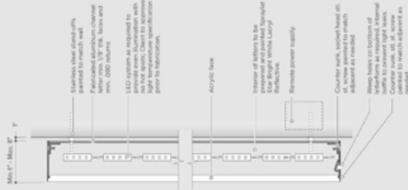
A Detail Section - Acrylic Face Intensely Illuminated Channel Letter Scale: NTS
